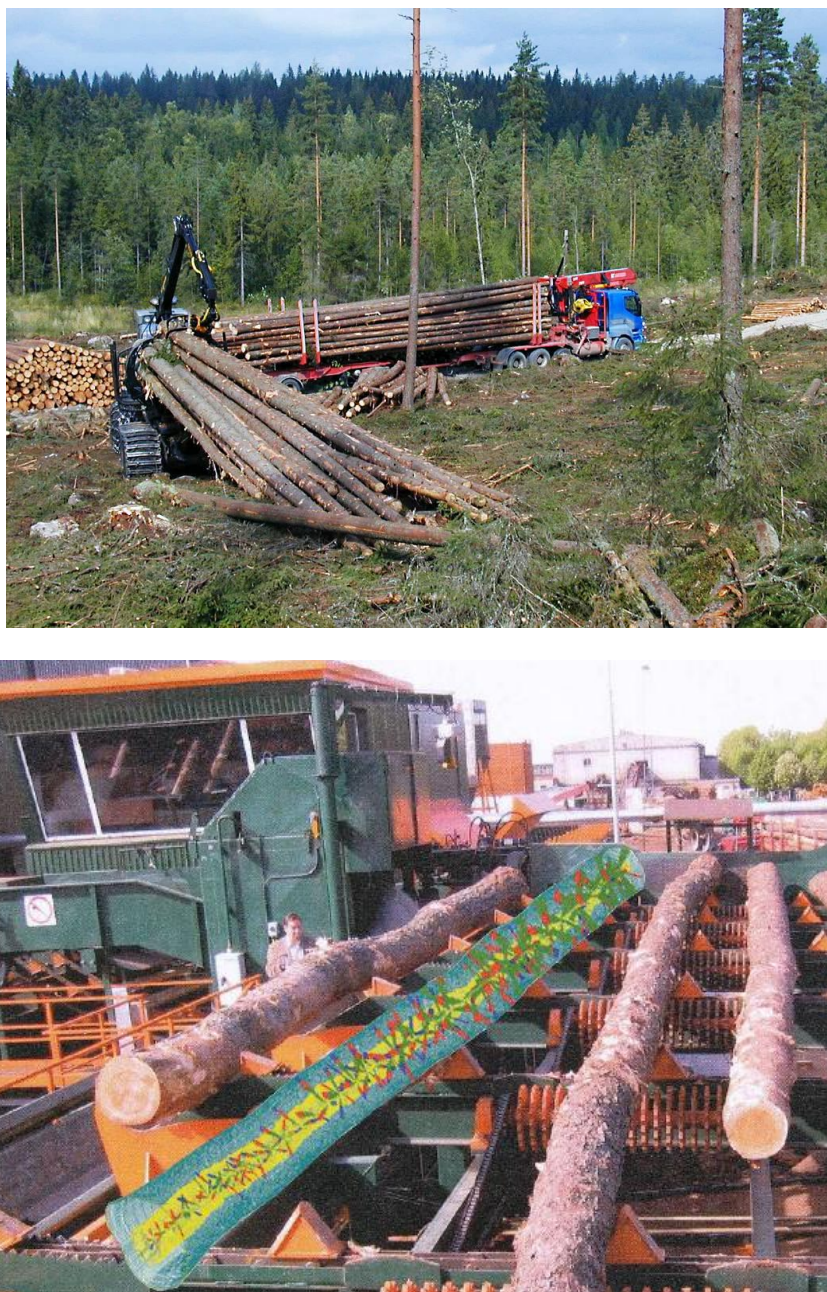
Figure 2. Transportation of stem parts (above) and stem terminal for cross cutting of parts.
