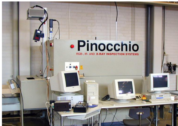
Figure 41. VTT's multisensor scanning is a powerful tool generating data of wood properties.
