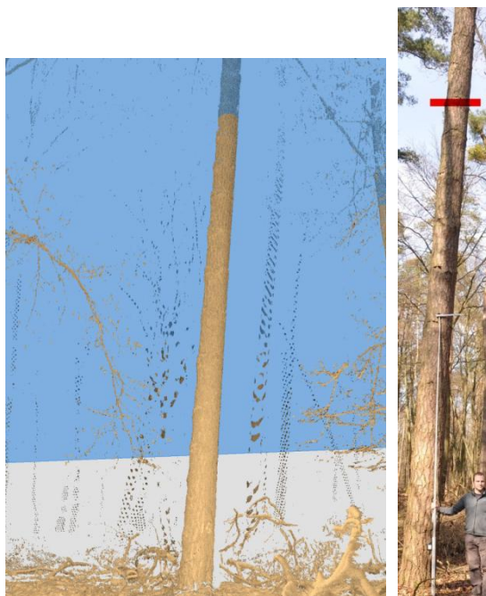
Fig. 17 Example of a medium to bad quality PNSY tree (quality 4) (2356_16): TLS point cloud visualization (left) and photograph (right)
